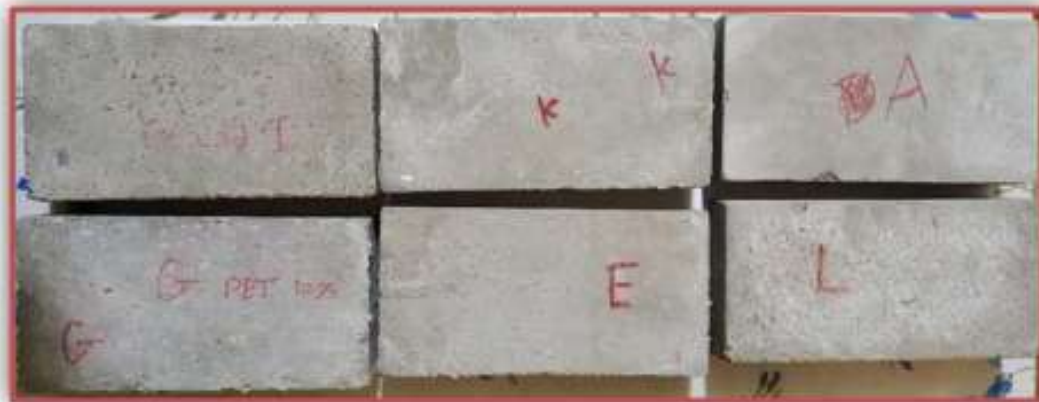
Fig (2) Cement Products with different weight percentages of PET waste after casting and drying
