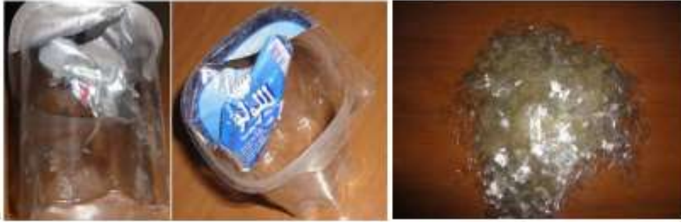
Fig. 1. (a) Polyethylene terephthalate (PET) waste cup before cutting (b) polyethylene terephthalate (PET) after cutting.
